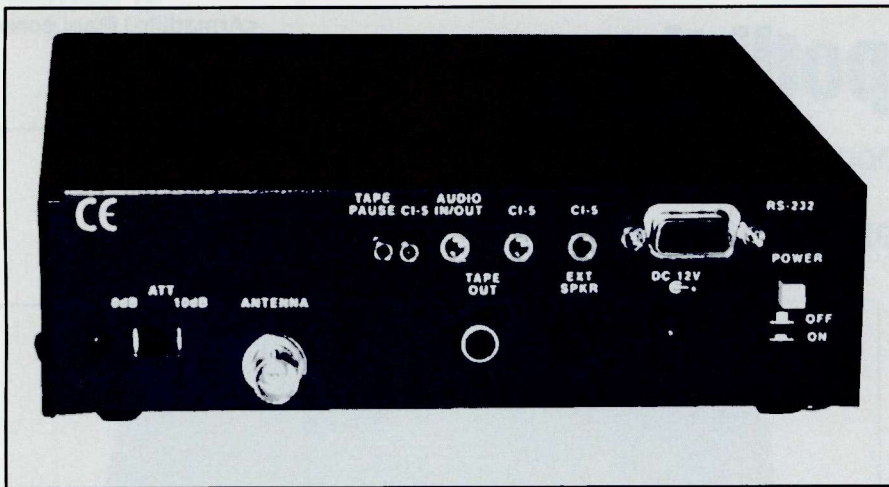
Lots of connections here. Note the 10-dB attenuator at the left and both conventional computer connections and CI-5. This may provide for lots of expansion in the future.
