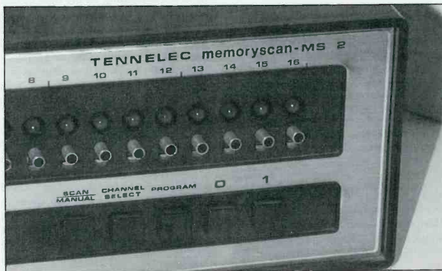
Early programmable radios include this Tennelec MS-2. This second generation portable was programmed with the 0 and 1 buttons from a code book. It took a while to reprogram, but didn't cost $5 every time you wanted to change one of its 16 frequencies.
